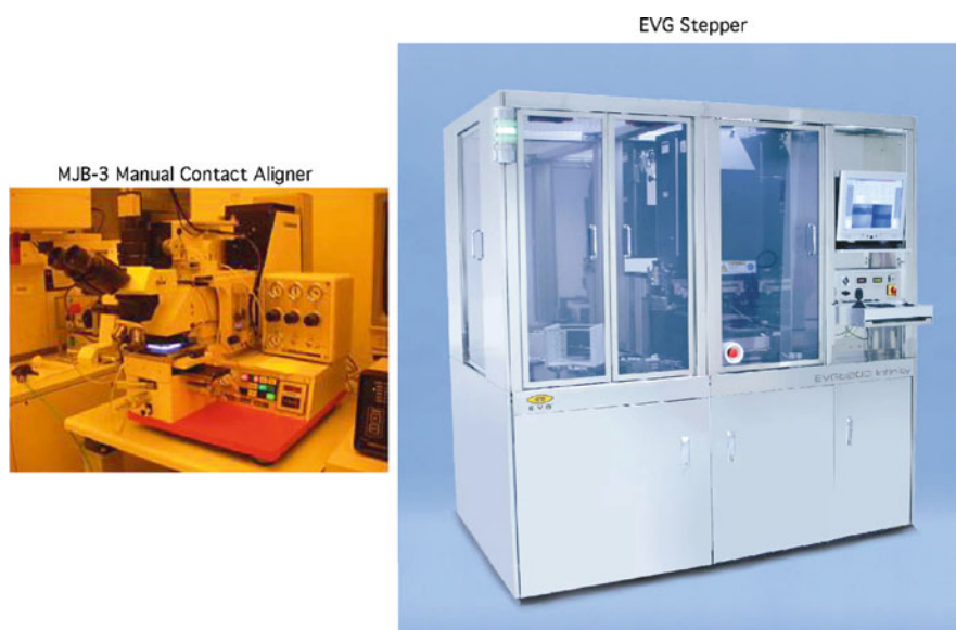
Fig. 9.10 Optical lithography systems: Manual contact aligner (left) and stepper (right) (Aligner reprinted courtesy of SUSS MicroTec Lithography GmbH, stepper reprinted courtesy of EV Group, Inc.)
